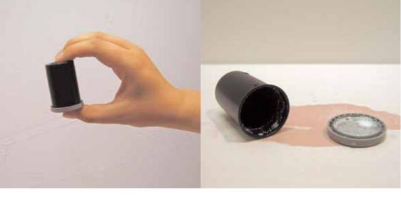
The Alka-Seltzer tablet reacts with the water and produces a gas called carbon dioxide or CO2. Pressure builds up in the canister as more gas is released, and the lid is eventually forced off. Sir Isaac Newton's third law of motion states, 'For every action there is an equal and opposite reaction' and this demonstration demonstrates it clearly: the lid pushes down against the desk, and the canister pushes upwards in the opposite direction, shooting off into the sky!
