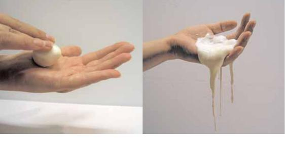
The cornflour does not dissolve in the water – it creates a suspension called a colloid. The cornflour particles are very fine and roll over each other which means that the mixture acts like a liquid. However, when energy is added to the mixture (by stirring or rolling in the hand) the particles of cornflour lock together and the water between the particles is pushed out of the way, so the slime behaves like a solid.
